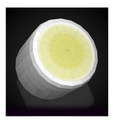
The outer bands of the refill matrix are constructed to produce areas of higher capillary pressure. The action pulls the liquid from the center of the refill towards these outermost areas.
